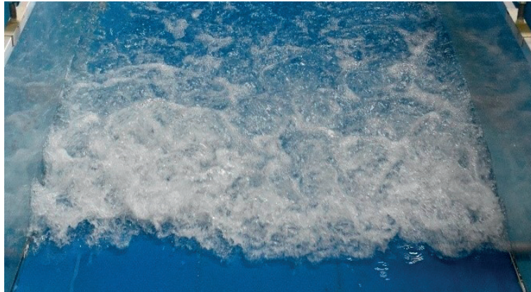
Figure 4.7 – Wet bed bore with d_0 = 0.82 m and initial still water depth h_0 = 0.03 m (test 4.8)
